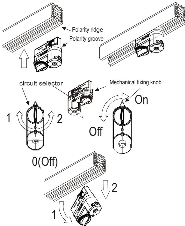
1. The fixture adapter is inserted with the polarity groove towards to the polarity ridge on the track
